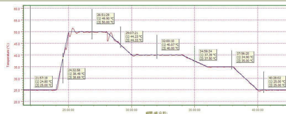
▲ Multi-stage (segment) climate simulation capability
